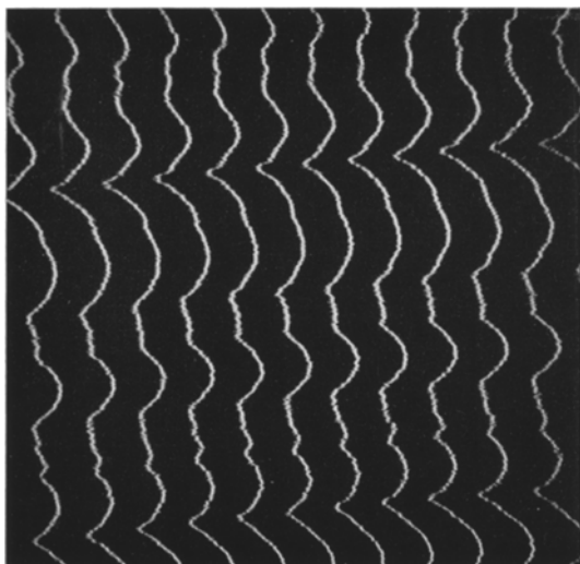
Figure 5 Graphical display of the cathodoluminescence intensity along a number of vertical scans of the platelet of fig. 4.
